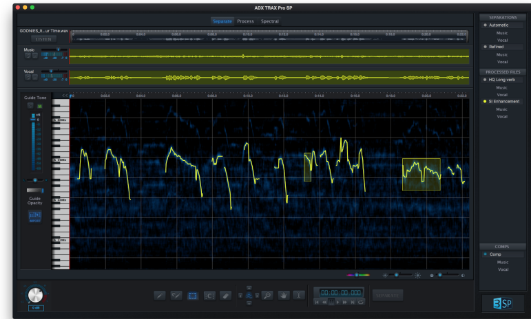
The Separate Screen displaying the SI Enhancement track with a new Music / Vocal balance (vocal down 10 dB).
